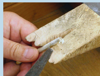
File the rough ingot to remove any flanges, pits or imperfections.
