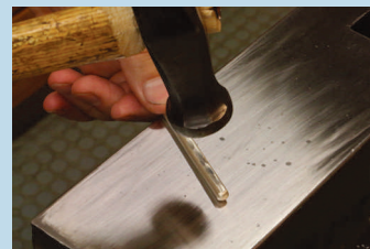
Lightly forge the ingot to harden the surface. Do five courses of forge, anneal, pickle.
